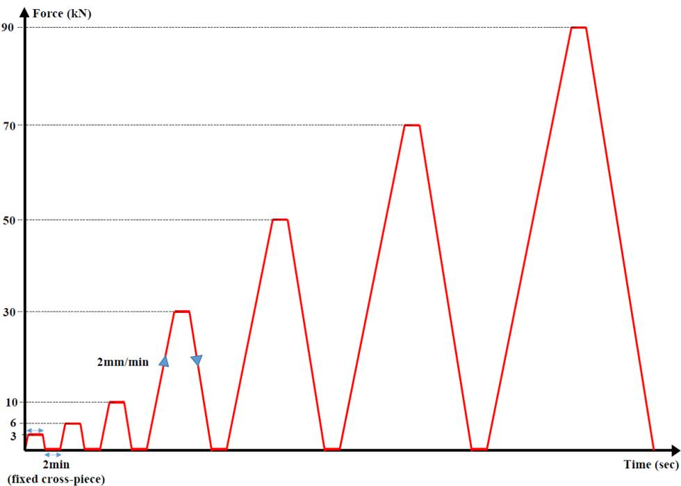
Figure 2: Schematic representation of the mechanical loading profile
