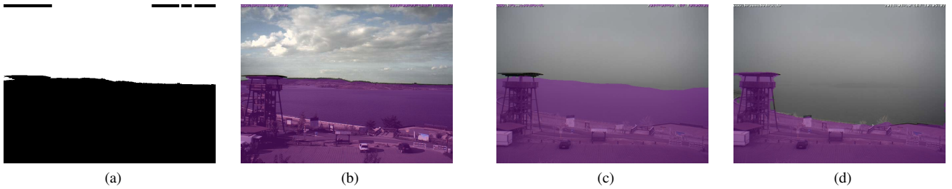
Fig. 2: Exemplary output on SkyFinder [13]: (a) shows the ground truth label for all images of camera 4801, (b) and (c) show segmentation results of two corresponding training images, and (d) shows segmentation results of a model trained on ADE20K. As can be seen in (b) and (c), the network that has been trained on SkyFinder memorizes the skyline.
