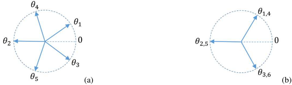
Fig. 16 Interleaving issue when phase differences are equal to 2/N : a) N odd case ( N = 5 ), b) N even case ( N = 6 ).
