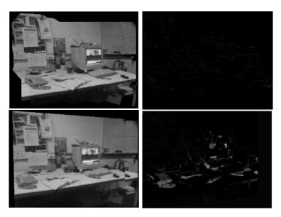
Figure 12: An example of image registration with several planes (top line) compared with image registration with one plane (bottom line). The left column represents the rectified frame after the compensation and the right column represents the disparity. Source: Images from Jin et al. [345].
