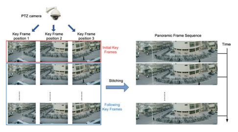
Figure 6: An example of a technique to construct a panoramic background model. Source: Images from Xue et al. [239].
