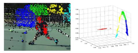
Figure 9: An example of clustering trajectories into a subspace (right) and the result on the image (left).
