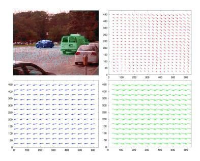
Figure 10: An example motion segmentation on the top left image. The three other images represent the optical flow of the three motions observed in the image. *Source*: Images from Zhu and Elgammal [326].
