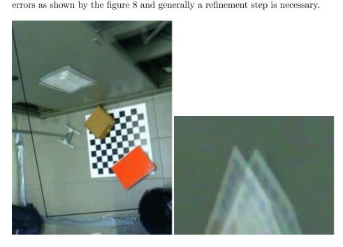
Figure 8: An example after image registration with a homography. The 2D transformation is based on the floor and we observe that the closet is misaligned. The second picture clearly shows this misalignment on the sheet paper. Source: Images from Romanoni et al. [282].
