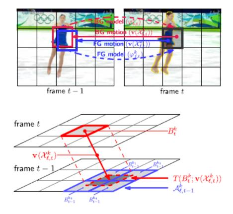
Figure 13: An example of a technique to divide the image into a regular grid and compensate the motion by blocks.
