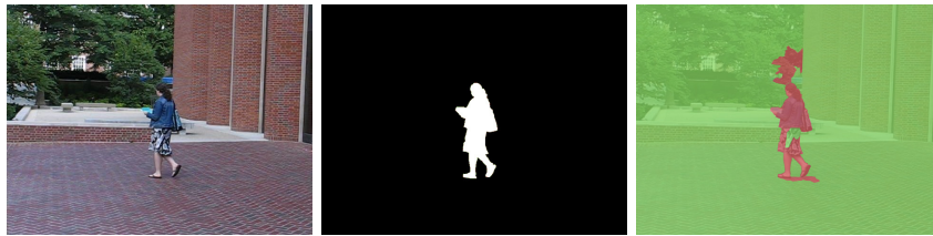
Figure 15: An example of background/foreground segmentation on the people01 sequence the from the Hopkins dataset. Left: the original image. Center: the ground truth. Right: an example of background/foreground segmentation where green pixels are labeled as background and red pixels are labeled as foreground.
