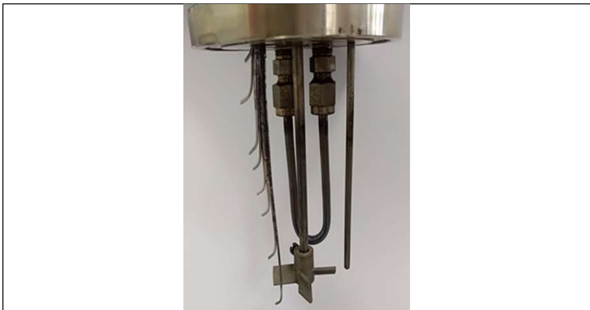
Figure 3: Photo of the instrumented head (b) showing the array of thermocouples, the stirring propeller, the regulation thermocouple and the internal cooling coil.
