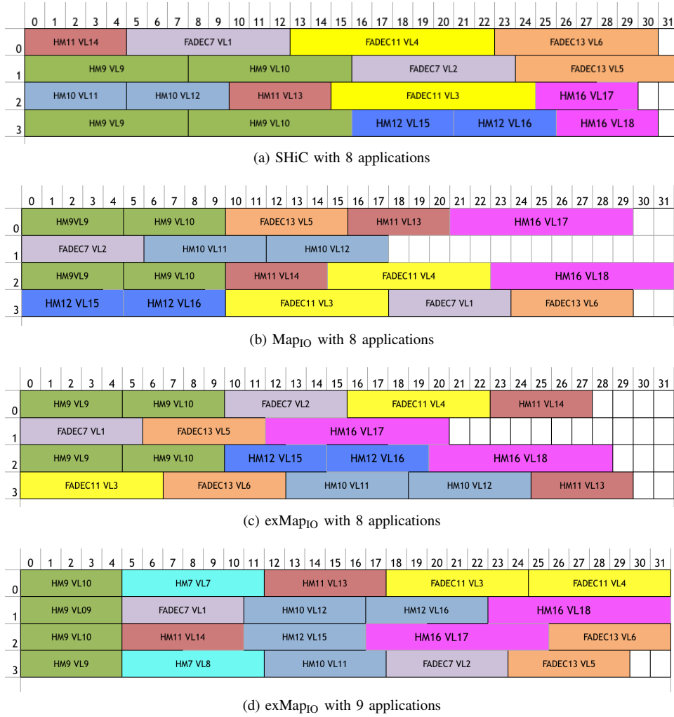
Fig. 7: Resulting scheduling tables for SHiC, MapIO and exMapIO with 8 applications and for exMapIO with 9 applications.
