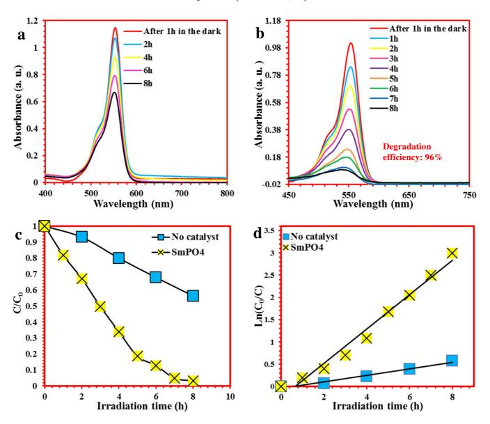
Fig. 5. (a) stability of the rhodamine B under UV light, (b) UV-vis absorption with time irradiation of a solution containing 100 mg  $SmPO_4$  and a 5ppm of rhodamine B, (c) Photodegradation of RhB in SmP suspension under UV-visible light (initial concentration of RhB, 5 mg/L). (d) pseudo-first-order kinetics of the photocatalyst.
