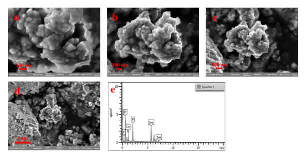
Fig. 2. SEM images and EDX spectrum of samarium phosphate SmPO<sub>4</sub> treated at 900  $^{\circ}\text{C}.$
