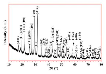
Fig. 1. XRD pattern of samarium phosphate  $SmPO_4$  calcined at 900  $^{\circ}C.$
