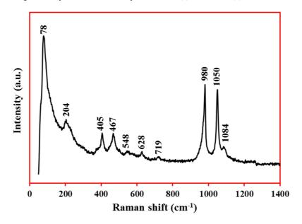
Fig. 4. Raman spectrum of SmPO<sub>4</sub> sample.
