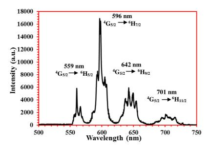
Fig. 6. Experimental emission bands of the SmPO<sub>4</sub> polycrystalline phase.
