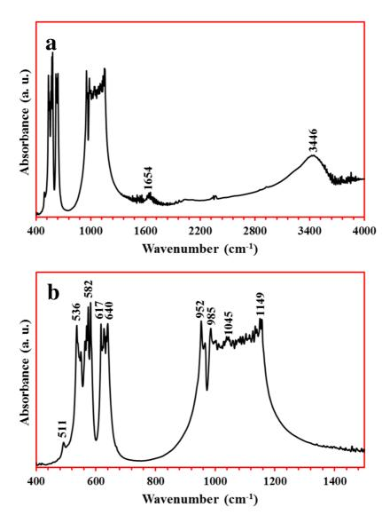
Fig. 3. FTIR spectrum of SmPO $_4$  nanoparticle between (a) 400-4000 and (b) 400-1400 cm $^{-1}$ .
