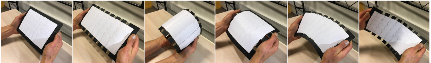
Figure 1: Six example shapes of a BEXHI prototype: a tablet that can be expanded and bent in 2 dimensions.
