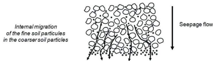
Figure 6: Principle of suffusion [Sharp et al., 2013]
