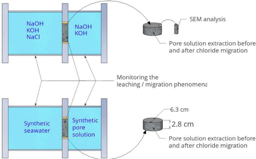
**Fig. 1.** Schematic representation of the two migration test protocols and material sampling for the investigation of the global ionic transport.
