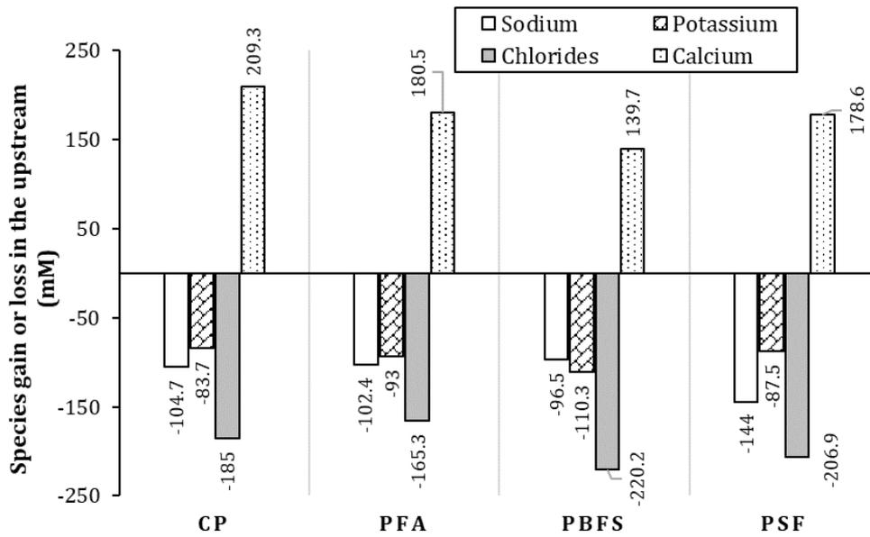
Fig. 7. Ion concentration gain or loss at the upstream at the end of the migration test.
