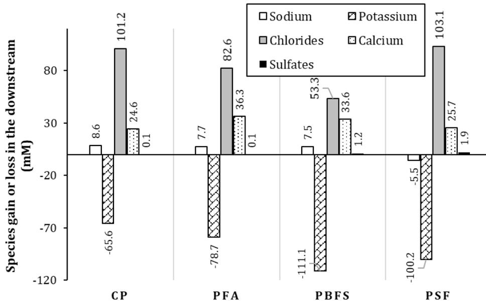
Fig. 8. Ion concentration gain or loss at the downstream at the end of the migration test.
