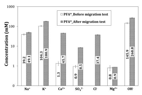
**Fig. 13.** Chemical composition of FA30\* pore solution before and after the migration test.
