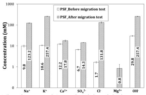
Fig. 6. Chemical composition of PSF pore solution before and after the migration test.
