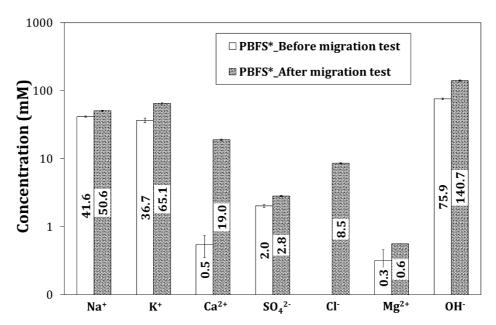
Fig. 14. Chemical composition of PBFS\* pore solution before and after the migration test.
