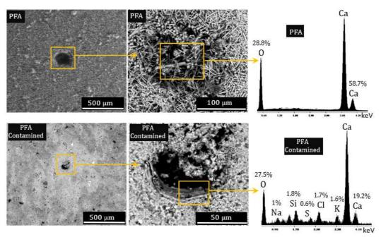
**Fig. 10.** SEM images and EDX spectra of PFA with and without chloride contamination.
