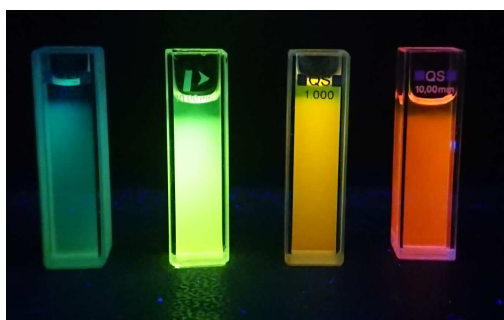
Figure 3: n -heptane solution under UV lamp irradiation (from left to right: 7b , 8b , 7a , 8a ) c = 1-3 \times 10^{-5} M. Photographs were taken in the dark upon irradiation with a hand-held lamp ( \lambda_{em} = 366 nm)
