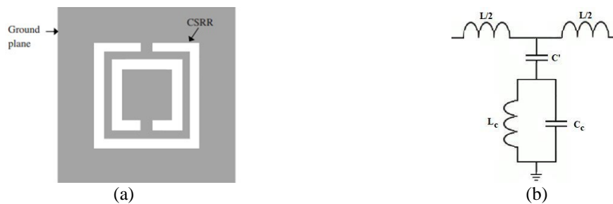
Figure 1. (a) Geometry of a CSRR unit cell, (b) Lumped-element equivalent circuit of the CSRR
