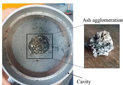
Figure 11. Ash agglomeration at the bottom of the conical cavity.
