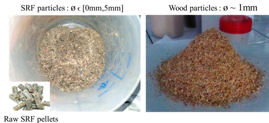
Figure 2. SRF and wood samples preparation.
