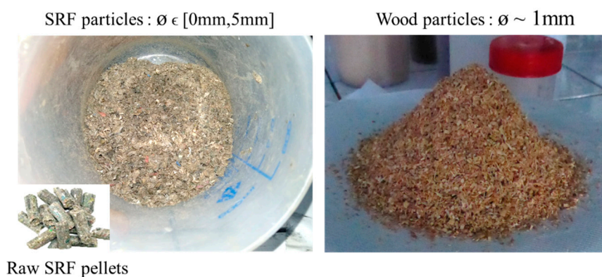
Figure 2. SRF and wood samples preparation.
