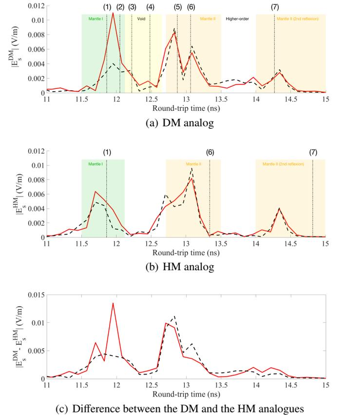
**Fig. 7.** Scattered fields for the DM and the HM analogs in the configuration described in Fig. 2 for  $\phi\phi$  polarization and the central transmitter–receiver position (Fig. 2). Measurement is in (–) and calculation in (– –). A Ricker window centered at 6.00 GHz is used. The vertical lines (1)–(6) shown in (a) and (b) correspond to the time points of interest, whose spatial correspondence is shown in Fig. 4 and Table 3.
