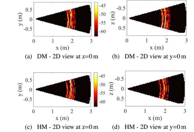
**Fig. 3.** 2D view of the 3D radargram obtained considering all the measurements in the configuration described in Fig. 2 for the two analogs, DM and HM. The distance corresponds to the two-way travel after a time-distance conversion considering a propagation in vacuum. The entire frequency band (2–18 GHz) was used for this radargram. The magnitude of the scattered field is given in decibels.
