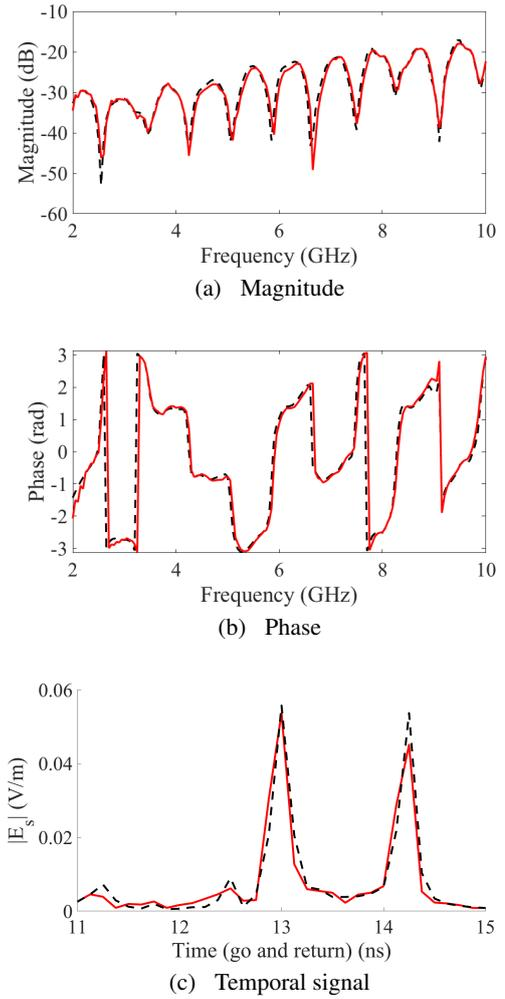
**Fig. 5.** Scattered field of the cube in the configuration described in Fig. 2 for  $\phi\phi$  polarization and the central transmitter–receiver position. Measurement is in (–) and calculation in (–). In the case of (c), the signal in the time domain was obtained using the inverse Fourier transform (Eq. (7)) and a Ricker window centered at 6.00 GHz.
