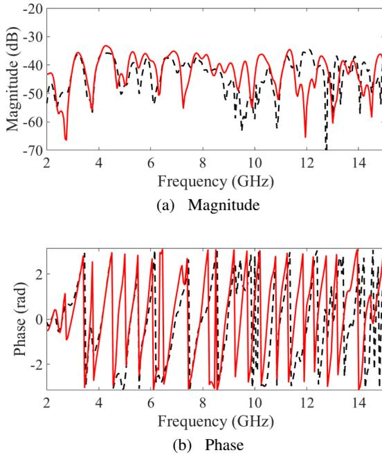
**Fig. 6.** Scattered field for the DM analogs in the configuration described in Fig. 2 for  $\phi\phi$  polarization and the central transmitter–receiver position (Fig. 2). Measurement is in (–) and calculation in (– –). The phase shown is the phase of the field after compensating the propagation distance.
