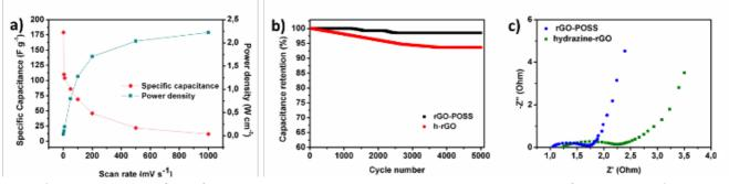
**Fig. 5** a) The dependence of specific capacitance and power density at various scan rates values for rGO-POSS. b) Cyclic stability of electrodes at 100 mV s<sup>-1</sup> for rGO-POSS and h-rGO c) comparison of Nyquist plots for rGO-POSS and hydrazine reduced graphene oxide.
