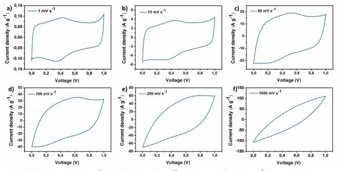
Fig. 4 Cyclic voltammetry curves of rGO-POSS electrode at different scan rates (1-1000 mV s<sup>-1</sup>).
