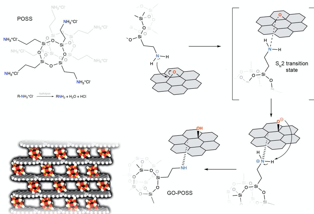
**Fig. 1** Scheme representing the mechanism of functionalization of GO with octaammonium POSS.
