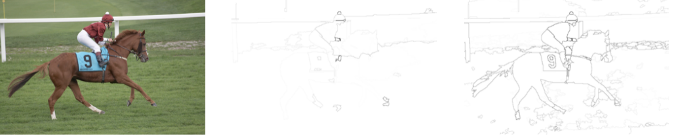
Fig. 1: (Left) original image extracted from the Pascal VOC 2010 dataset, and the saliency maps (an equivalent representation of hierarchical segmentation) resulting from the HGB method using the original observation scale (middle) and from one of our proposed observation scale selection strategies (right). A video version of this illustration showing the successive levels of the hierarchy is available at www.tobeinsertedByPRLwhenAvailable.com .
