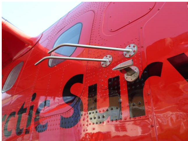
Figure A1. Photo of the rear-facing chemistry inlets on the BAS Twin Otter aircraft.
