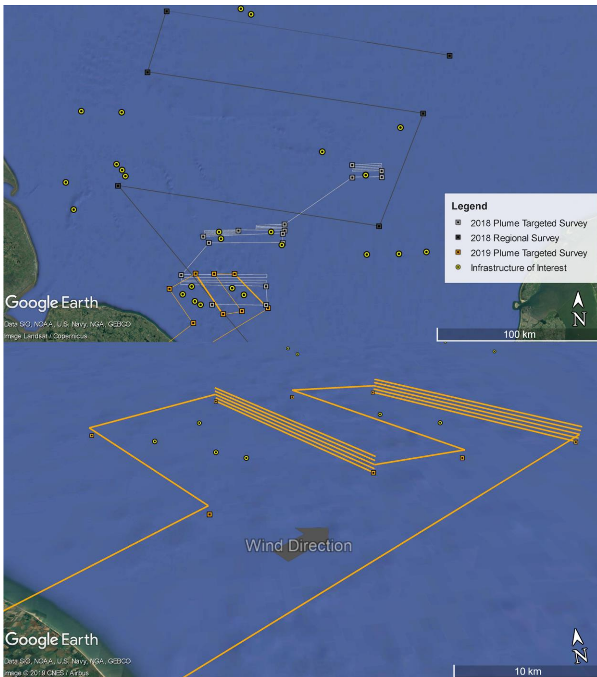
Figure 3: [top panel] flight patterns showing the regional and plume capture styles of flight deployed between 2018 and 2019, alongside infrastructure of interest (such as drilling rigs, gas distribution platforms or production platforms). [bottom panel] a 2019 plume sampling survey showing idealised stacked transects in the 2D plane downwind of infrastructure of interest.
