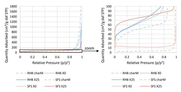
Figure 8 |  $N_2$  adsorption isotherms of rice husk and sunflower seed shell chars at several pyrolysis and gasification conversions.
