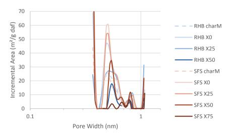
Figure 11 | Ultramicropore size distribution using DFT model from  $CO_2$  adsorption isotherms of rice husk and sunflower seed shell chars at several pyrolysis and gasification conversions expressed in terms of incremental area.
