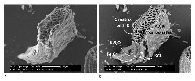
Figure 16 | SEM image of a char particle from SFS\_X25 with a. SE detection and b. BSE detection.
