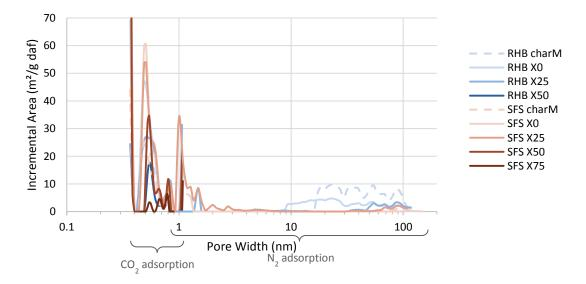
Figure 10 | Pore size distribution using DFT model from  $N_2$  and  $CO_2$  adsorption isotherms of rice husk and sunflower seed shell chars at several pyrolysis and gasification conversions expressed in terms of incremental area.
