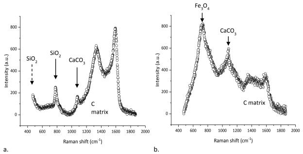
Figure 19 | Raman spectra showing inorganic compounds of the sample a. RHB\_X100 and b. SFS\_X75.
