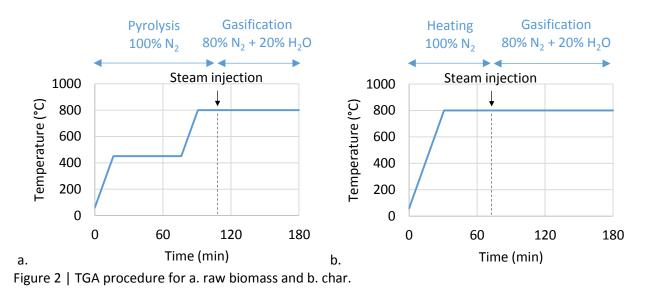
In the case of raw biomass (Figure 2a), the procedure described by Hognon *et al.* (Hognon et al., 2014) was applied to a mass of approximately 15 mg to be in chemical regime (Dupont et al., 2011).
