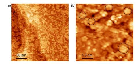
**Figure 2.** STM images corresponding to phosphorus adlayer deposited on Au(111) at RT. (a) phosphorus adlayer on Au(111), revealing a rough surface morphology with high surface coverage ( $150 \times 150 \text{ nm}^2$ , U = 1.0 V, I = 1.0 nA). (b) Atomic resolution STM image of phosphorus adlayer on Au(111) ( $6.5 \times 6.5 \text{ nm}^2$ , U = 930 mV, I = 1.1 nA). The P-clusters of different geometrical shapes are highlighted by black dashed circles.
