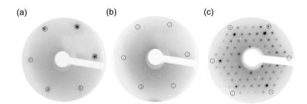
**Figure 1.** LEED patterns recorded at 57 eV. (a) bare Au substrate, (b) after deposition of phosphorus on Au(111) at RT, (c) after post-annealing at 530 K for 30 min. The  $(1 \times 1)$  spots of Au(111) substrate are highlighted by black circles in all the images.
