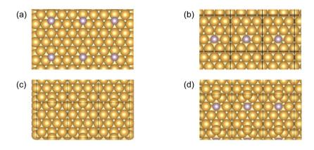
**Figure 4.** Configurations considered in the calculation of the total energy: (a) Au(111) surface with a P atom adsorbed on an *fcc* site, (b) a P atom replacing a Au surface atom, (c) a Au atom adsorbed on an *fcc* site with no P atom on the surface, and (d) a P atom replacing a Au surface atom with a Au atom adsorbed on a neighboring *fcc* site.
