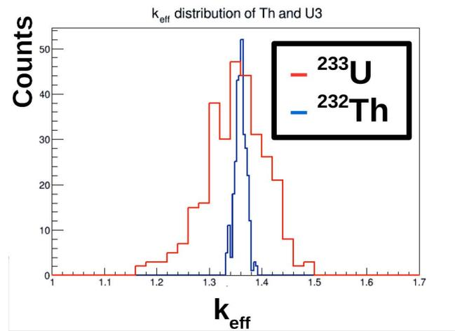
**Figure 3.** (color online)  $k_{eff}$  distribution obtained for PWR assembly calculations, varying the <sup>233</sup>U evaluation in red and the <sup>232</sup>Th in blue.
