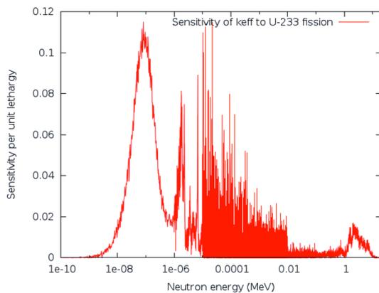
**Figure 5.** (color online)  $k_{eff}$  sensitivity to  $^{233}\text{U}(n, f)$  reaction.
