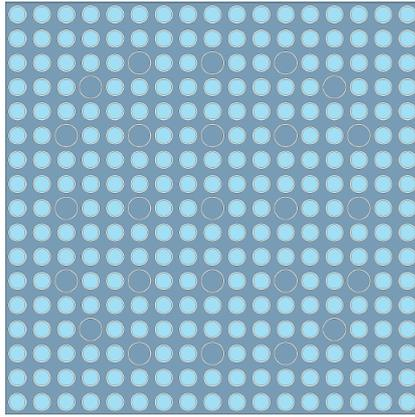
**Figure 1.** (color online) PWR Assembly geometry. Zirconium sheath (white), TH/VO<sub>2</sub> fuel (blue), light water (grey).
