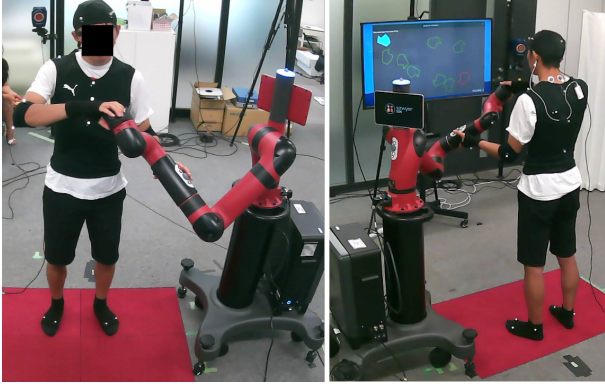
Fig. 2: The user uses the robot as a joystick to play the visual puzzle game.
