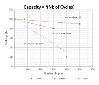
Fig. 5. Characterisation of the battery module lifetime
