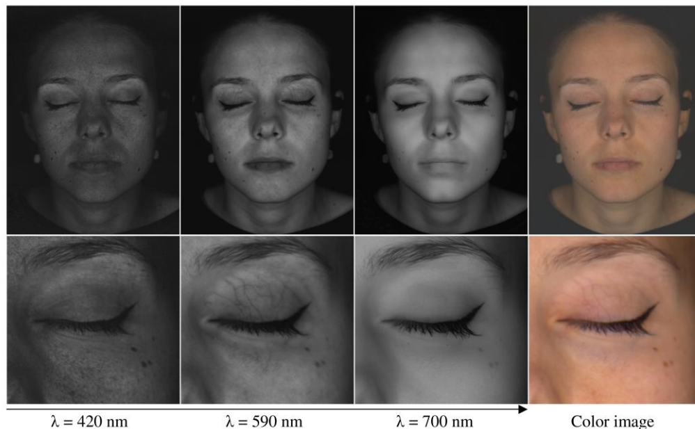
Figure 3. Hyperspectral image at several wavelengths and corresponding color image. Full face image (top), detail of right eye (bottom).
