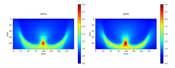
Figure 2: Experimental (EBT3 gafchromic film - left) and simulated (GATE - right) dose maps of a VMAT plan. Dose maps are normalized by the mean dose value of the slice.
