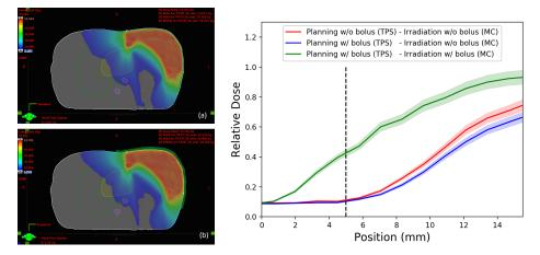
Figure 6: Left: TPS dose maps for VMAT planning without (a) and with a 5 mm bolus (b); Right: Monte Carlo calculations of percentage depth dose distributions (breast) for different planning (TPS) and irradiation (MC) configurations: planning and irradiation without bolus (red), planning with a 5 mm bolus and irradiation without bolus (blue), planning and irradiation with a 5 mm bolus (green). The dashed line represents the position of the first voxel of the phantom.
