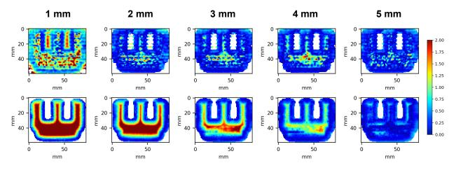
Figure 5: 2D-gamma index distributions (4%/3mm) for GATE (top) and TPS (bottom) calculations with respect to experimental (EBT3) dose maps for a static IMRT plan irradiation for various depths.
