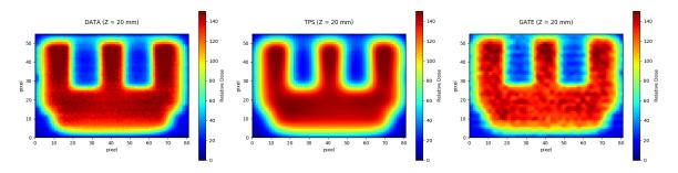
Figure 4: Experimental (EBT3 films - left), TPS (Eclipse AAA - center) and Monte Carlo (GATE - right) 2D dose maps at 20 mm for a static IMRT plan irradiation. Mean dose values are used for normalization.
