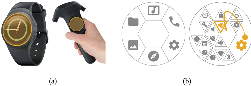
Fig. 10. SCM adapts to various device shapes. (a) Examples of small round touch-sensitive surfaces integrated in a smartwatch and a VR controller (highlighted in orange). (b) Examples of SCM layouts using hexagonal cells better suited for round surfaces.
