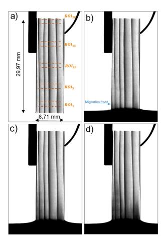
Fig. 6. Water uptake in spruce along longitudinal direction at  $t_0(a)$ ,  $t_{50s}(b)$ ,  $t_{4h01}(c)$  and  $t_{23h18}(d)$
