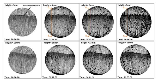
Fig. 8. Cross section located at 5 (top) and 15 mm (bottom) from liquid contact water during imbibition
