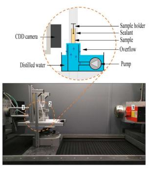
Fig. 1. General view of the experimental setup inside the tomograph: (1) CCD detector, (2) sample holder with water system supply and (3)  $\mu$ X-ray source.
