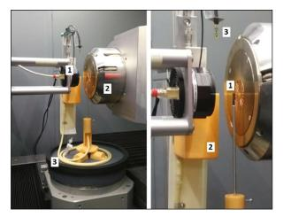
**Fig. 2.** Experimental setup for 3D imaging with a general view on the left with CCD detector (1), nano X-ray source (2) and flexible tube (3). On the right, a zoom of the sample positioned at the top of aluminium tube (1), a water container (2) and a SHT75 sensor (3).
