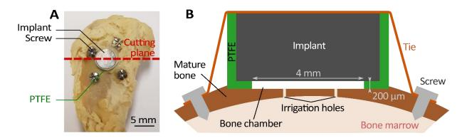
Figure 1 : A) Coin-shaped implant inserted into the proximal-medial part of a rabbit tibia, B) Schematic cross-section of the coin-shaped implant model
