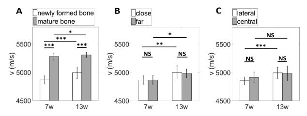
Figure 6 : Distribution (average and standard deviation values) of the wave velocity v after 7 weeks (7w) and 13 weeks (13w) of healing time. A: mature vs newly formed bone tissue, B: close vs far groups and C: lateral vs central groups. The Mann-Whitney U-test analysis leads to: \* = p-value  $\le 0.05$ , \*\* = p-value  $\le 0.01$ , \*\*\* = p-value  $\le 0.001$ , \*\*\* = p-value  $\ge 0.001$ , \*\* = p-value
