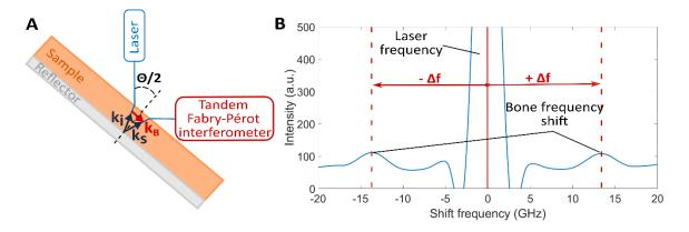
Figure 3 : A) Schematic representation of reflection induced  $\Theta$  angle (RI $\Theta$ A) micro-Brillouin scattering measurement configuration, B) Micro-Brillouin spectrum and bone frequency shifts (denoted by  $\Delta$ f). The spectrum represents the filtered (1D median filter) and smoothed data for one given measuring point corresponding to a wave velocity equal to 4994 m/s.
