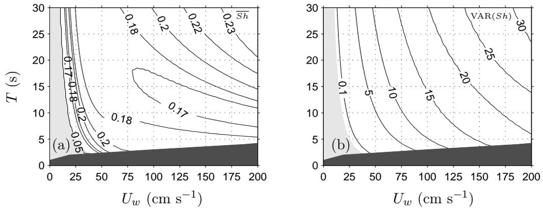
Figure 8: Isograms of (a)  $\overline{Sh}$ , and (b)  $\text{VAR}(Sh)$  showing dependences on orbital velocity  $U_w$  and wave period  $T$ . Dark grey delimits the unstable breaking waves ( $H < 0.8 D$ ) and light grey delimits the laminar regime ( $Re_\delta < 320$ ).
