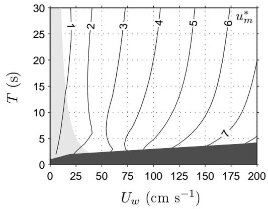
Figure 3: Maximum shear velocity  $u_m^*$  dependence on orbital velocity  $U_w$  and period  $T$  of the wave. Dark grey delimits the unstable breaking waves ( $H < 0.8 D$ ) and light grey delimits the laminar regime ( $Re_s < 320$ ).
