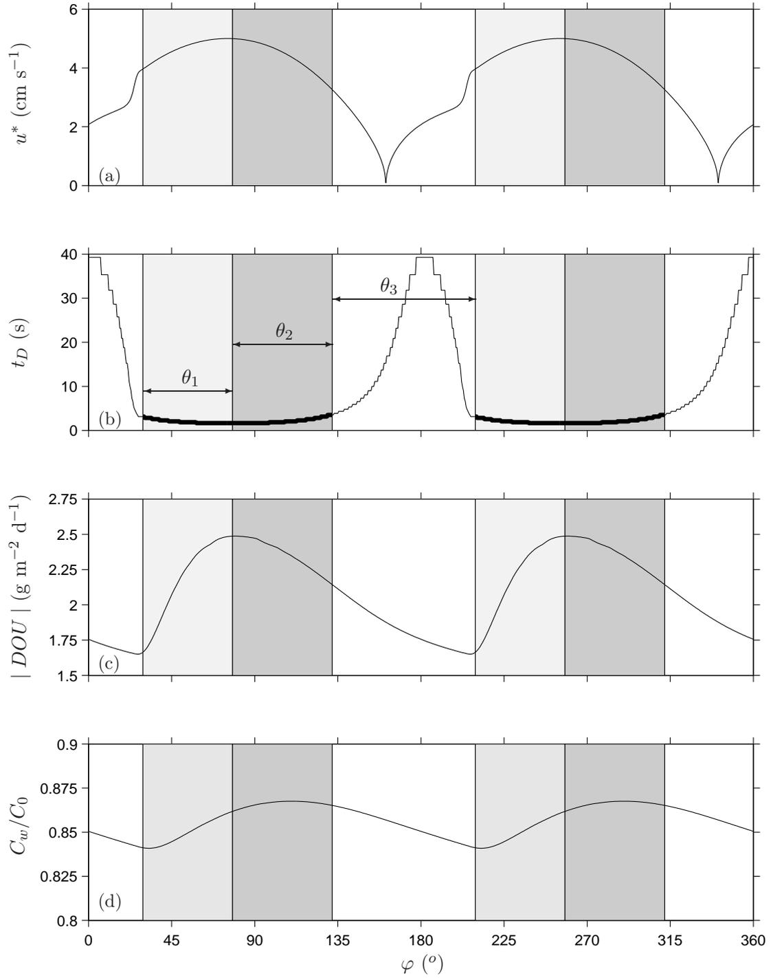
Figure 5: Temporal evolution of (a)  $u^*$ , (b)  $t_D$ , (c)  $DOU$ , and (d)  $C_w/C_0$  during a wave cycle, for  $u_m^*=5$  cm s<sup>-1</sup>,  $T=15$  s, and  $\mu=2000$  g m<sup>-3</sup> d<sup>-1</sup>. Light grey delimits the turbulent period  $\theta_1$  and dark grey delimits the turbulent period  $\theta_2$ .
