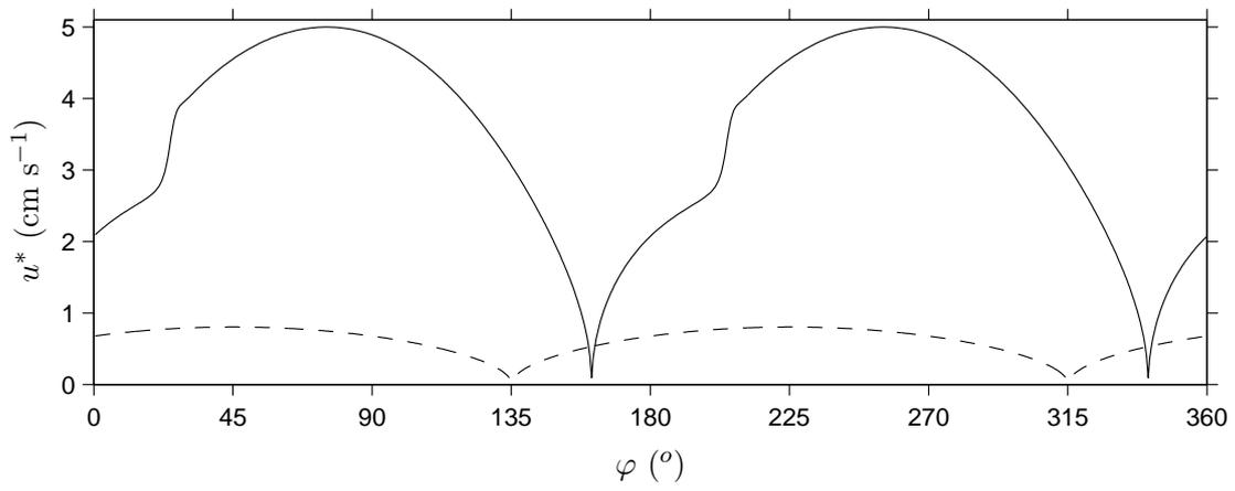
Figure 2: Shear velocity  $u^*$  during a wave cycle for  $T=15$  s, and  $u_m^*=5$  cm s<sup>-1</sup> (solid line),  $u_m^*=0.8$  cm s<sup>-1</sup> (dashed line).
