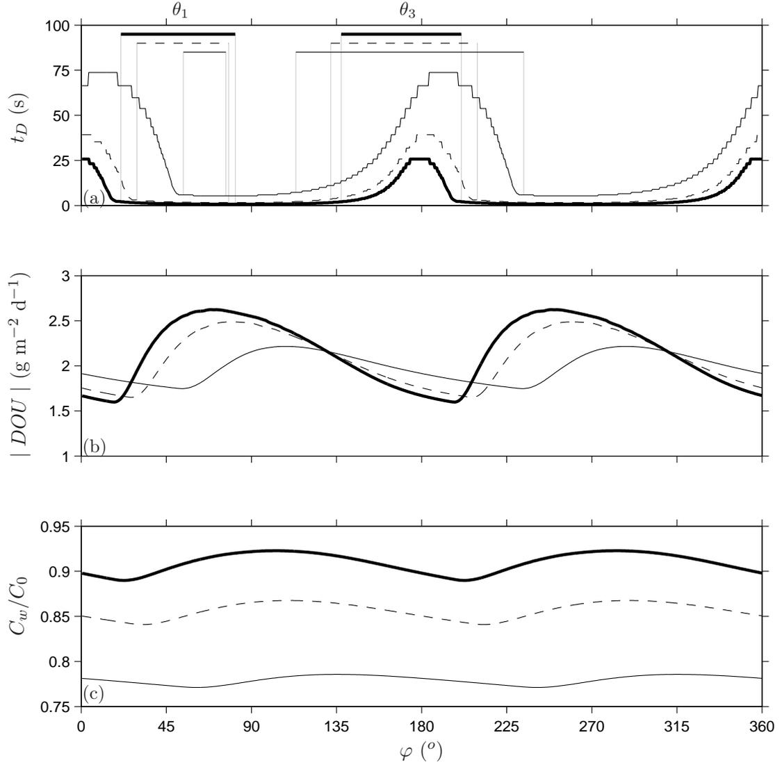
Figure 6: Temporal evolution of (a)  $t_D$ , (b)  $DOU$ , and (c)  $C_w/C_0$  during a wave cycle, for  $T=15$  s,  $\mu=2000 \text{ g m}^{-3} \text{ d}^{-1}$ , and  $u_m^*=3 \text{ cm s}^{-1}$  (solid line),  $u_m^*=5 \text{ cm s}^{-1}$  (dashed line),  $u_m^*=7 \text{ cm s}^{-1}$  (bold line).
