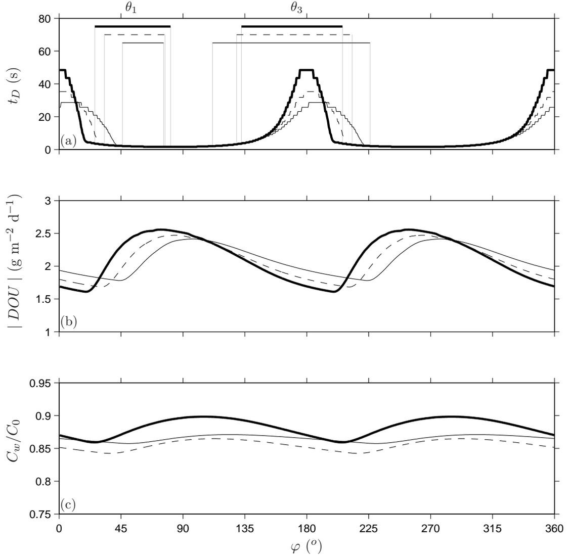
Figure 7: Temporal evolution of (a)  $t_D$ , (b)  $DOU$ , and (c)  $C_w/C_0$  during a wave cycle, for  $u_m^*=5 \text{ cm s}^{-1}$ ,  $\mu=2000 \text{ g m}^{-3} \text{ d}^{-1}$ , and  $T=7 \text{ s}$  (solid line),  $T=12 \text{ s}$  (dashed line),  $T=25 \text{ s}$  (bold line).
