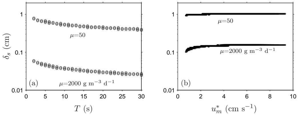
Figure 10: Penetration depth  $\delta_s$  dependence on (a) wave period  $T$  for the laminar regime ( $Re_\delta \leq 320$ ) and (b) maximum shear velocity  $u_m^*$  for the turbulent regime ( $Re_\delta > 320$ ), and the two biogeochemical activities tested.
