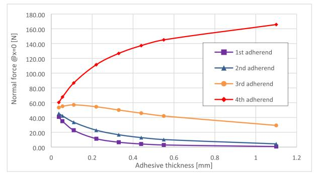
Fig. 18. Normal forces in the adherends vs. adhesive thickness.
