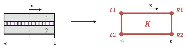
Fig. 4. Physical single lap model transformed into ME.
