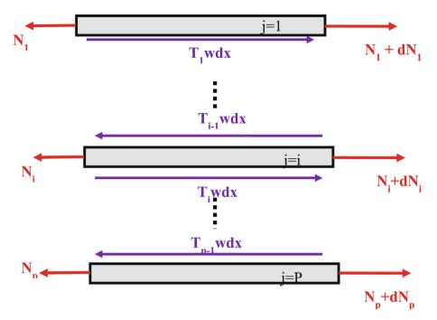
Fig. 12. Local equilibrium representation of multilayered bonded joint.
