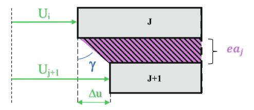
Fig. 2. Adherends relative displacement and shear angle presentation.
