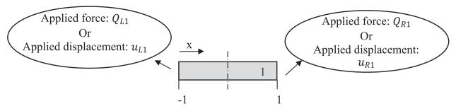
Fig. 5. Application of boundary condition at overlap ends.
