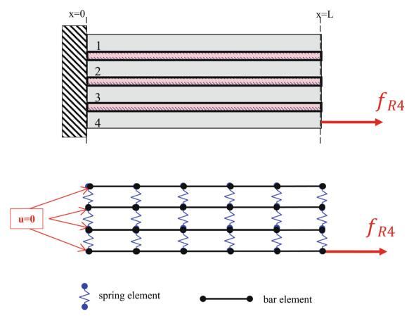
Fig. 14. Scheme of test 1 & 2 configuration.
