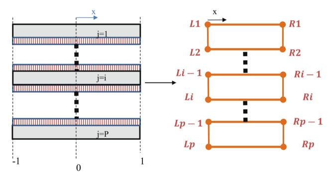
Fig. 13. ME representation of multilayered bonded joint.
