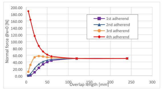
Fig. 20. Normal forces in the adherends vs. overlap length.
