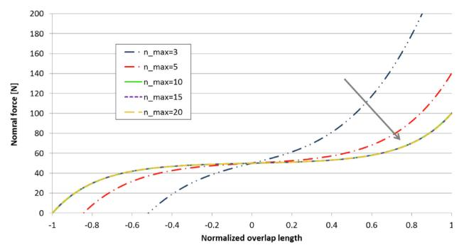
Fig. 8. Convergence of adherend normal force increasing  $n_{max}$ .
