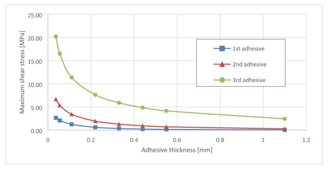
Fig. 17. Maximum shear stress vs. adhesive thickness.
