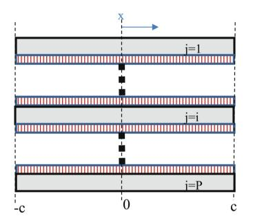
Fig. 11. Multilayered bonded joint configuration.
