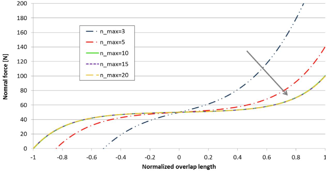
Fig. 8. Convergence of adherend normal force increasing  $n_{max}$ .
