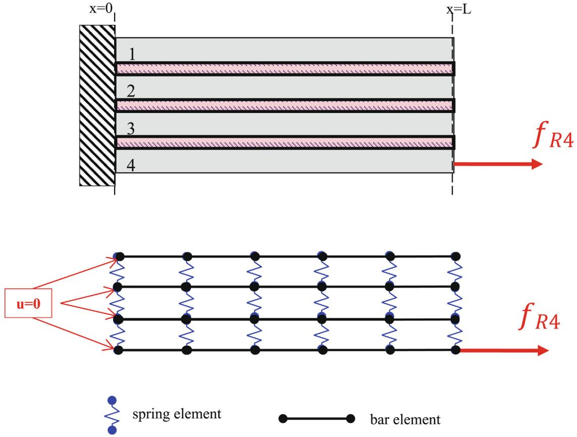
Fig. 14. Scheme of test 1 & 2 configuration.
