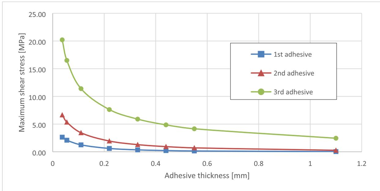
Fig. 17. Maximum shear stress vs. adhesive thickness.
