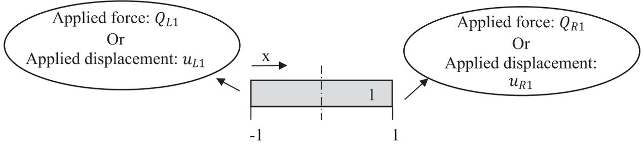
Fig. 5. Application of boundary condition at overlap ends.
