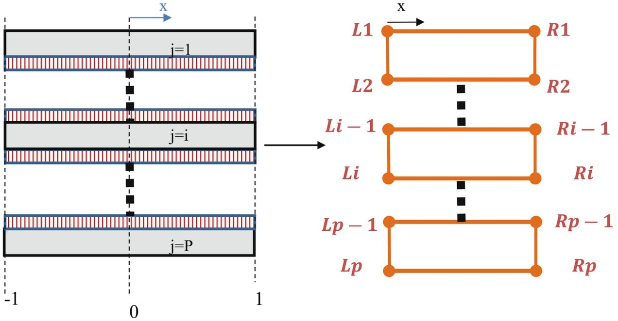
Fig. 13. ME representation of multilayered bonded joint.
