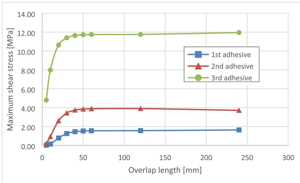
Fig. 19. Maximum shear stress vs. overlap length.
