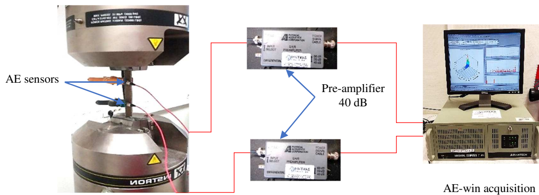
Fig. 3. Experimental setup of acoustic emission method.
