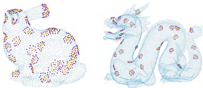
FIGURE 16 Contact points for the Stanford bunny and dragon. The applied loads simulating contact are centered on the orange dots and have an application range of two neighbors (graph distance), marked in the figure with yellow and violet colors [Color figure can be viewed at wileyonlinelibrary.com ]
