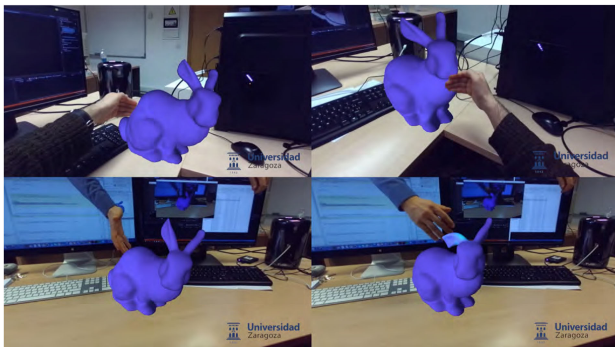
FIGURE 15 Some frames extracted from the bunny sequence. Colors show the stress map associated with the deformations imposed by contact with real objects [Color figure can be viewed at wileyonlinelibrary.com ]
