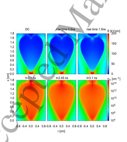
**Figure 9.** For a DC applied voltage and voltages with rise times of 0.5 and 1.5 ns and a voltage plateau of  $55 \,\mathrm{kV}$ : cross-sectional views of the absolute value of the electric field and electron density at the connection time at the cathode, i.e. at t = 2.1, 2.45 and 3.1 ns, respectively.
