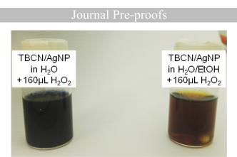
Fig. S5. Comparison between TBCN/AgNP prepared with the addition of 160  $\mu$ L of H<sub>2</sub>O<sub>2</sub> ( $\alpha = 0.33$ ) in a pure water medium or in a H<sub>2</sub>O/EtOH mixture. The presence of ethanol seems to affect the H<sub>2</sub>O<sub>2</sub> post-treatment since the color suspension did not turn blue like the pure water suspension.
