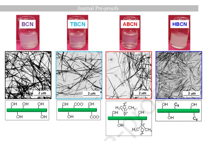
Fig. 1. BCN, TBCN, ABCN and HBCN suspensions: visual appearance (top line), STEM images (middle line) and scheme of various surface modifications (bottom line).
