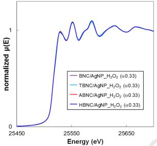
Fig. S7. XANES spectra of BCN-., TBCN-., ABCN-. and HBCN/ AgNP\_H<sub>2</sub>O<sub>2</sub> hybrids mixed with 160  $\mu$ L of H<sub>2</sub>O<sub>2</sub> ( $\alpha$  = 0.33).
