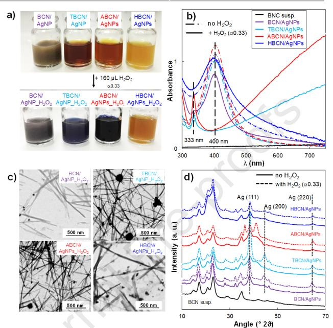
Fig. 5. (a) Color variation of hybrid suspensions; (b) UV-Vis spectra; (c) STEM images; (d) XRD patterns of BCN-, TBCN-, ABCN-, HBCN-/AgNP\_H<sub>2</sub>O<sub>2</sub> hybrid suspensions with the addition of 160  $\mu$ L of H<sub>2</sub>O<sub>2</sub> ( $\alpha$  = 0.33).
