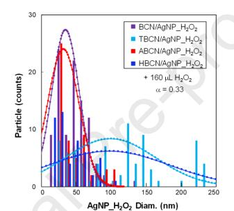
Fig. S6. Size distribution histograms of AgNPs\_ $H_2O_2$  in BCN-. TBCN-. ABCN. HBCN/AgNP\_ $H_2O_2$  hybrids at  $H_2O_2/AgNP$  ratios.  $\alpha$ , equal to 0.33.
