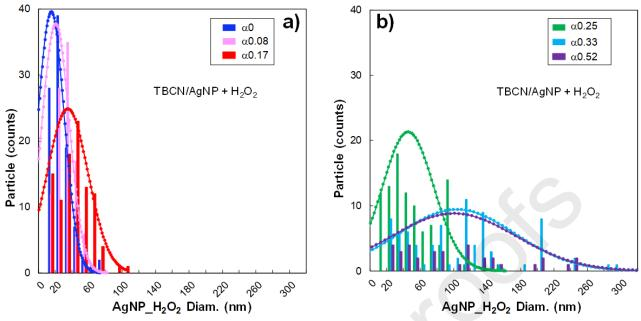
Fig. S3. Size distribution histograms of TBCN/AgNP\_H<sub>2</sub>O<sub>2</sub> hybrids with various volumes of H<sub>2</sub>O<sub>2</sub> added and, consequently, various H<sub>2</sub>O<sub>2</sub>/AgNP mass ratios.  $\alpha$ . from 0 to 0.17 (a), and from 0.25 to 0.52 (b).
