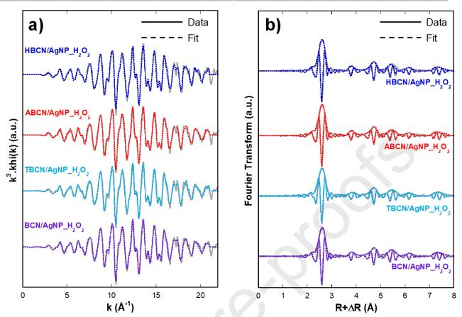
Fig. S8. (a) EXAFS spectra Fourier transform (solid gray lines) and fit (dotted lines); (d) magnitude and imaginary part (solid gray lines) and fit (dotted lines) of the Fourier transform of BCN-., TBCN-., ABCN-. and HBCN/ AgNP\_H<sub>2</sub>O<sub>2</sub> hybrids with 160 $\mu$ L of H<sub>2</sub>O<sub>2</sub> ( $\alpha$ = 0.33).
