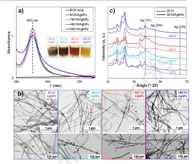
Fig. 3. Characterizations of BCN-, TBCN-, ABCN-, HBCN-/AgNP hybrid suspensions: (a) UV-Vis spectra; inset: sample pictures; (b) STEM images; (c) XRD patterns.
