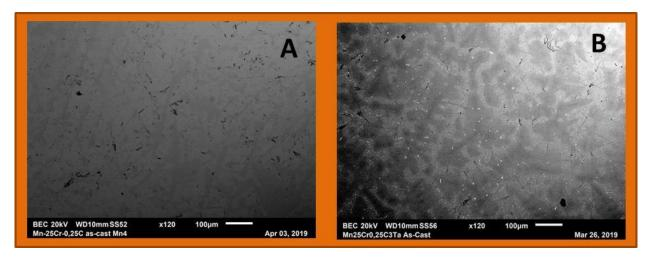
**Figure 2.** Microstructures of the MCC1 (A) and MCC1T (B) alloys (SEM/BSE mode, low magnification)
