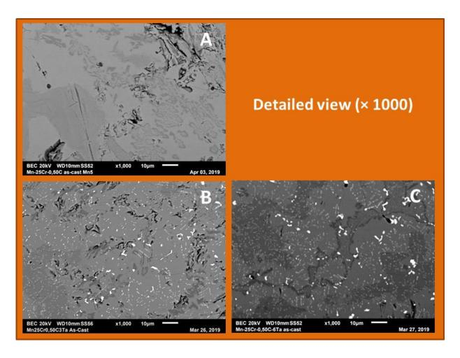
**Figure 5.** Microstructures of the MCC2 (A), MCC2T (B) and MCC2T' (C) alloys (SEM/BSE mode, high magnification)
