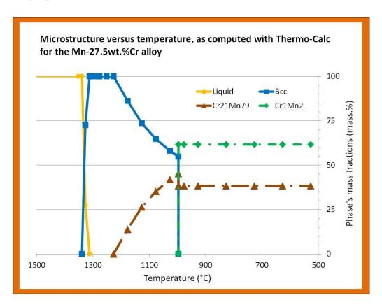
**Figure 8.** Phase transformations occurring for the MC alloy from 1500°C to 500°C: solidification and solid state cooling (computed by Thermo-Calc N with Wth KP database)
