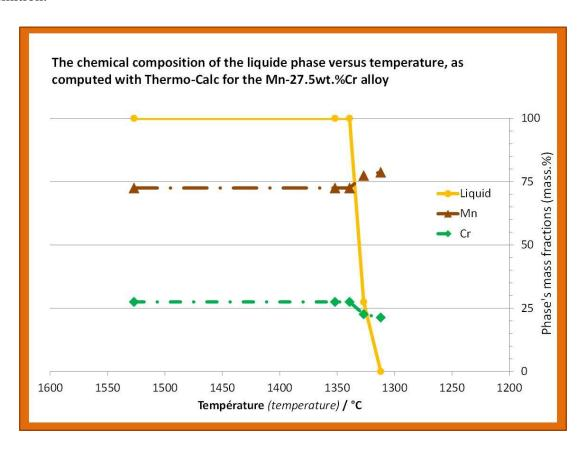
**Figure 9.** Evolution of the chemical composition of the liquid during the solidification of the MC alloy (computed by Thermo-Calc N with with KP database)
