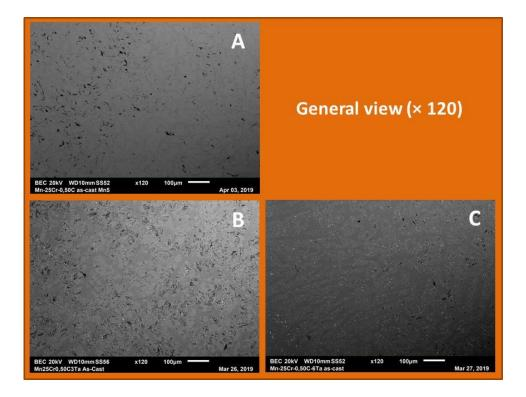
**Figure 4.** Microstructures of the MCC2 (A), MCC2T (B) and MCC2T' (C) alloys (SEM/BSE mode, low magnification)
