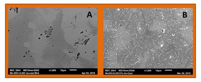
**Figure 3.** Microstructures of the MCC1 (A) and MCC1T (B) alloys (SEM/BSE mode, high magnification)
