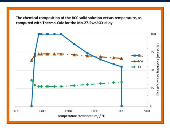
**Figure 10.** Evolution of the chemical composition of the BCC Cr solid phase, between its appearance at solidification start and its disappearance at the end of the peritectorial reaction, for the MC alloy (computed by Thermo-Calc N with with KP database)
