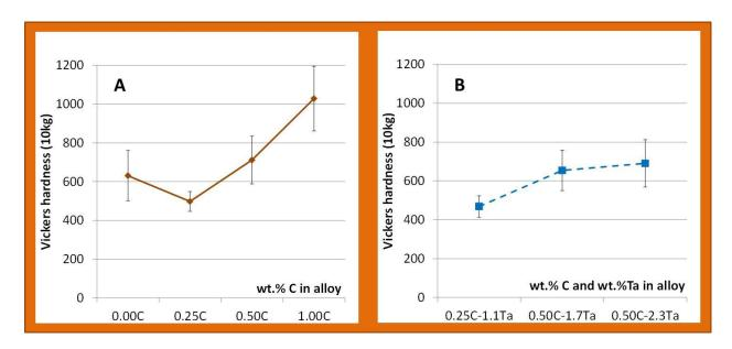
**Figure 7.** Hardness evolution versus the C content (A) and the C and Ta contents (B) (Vickers indentations under a 10 kg load)
