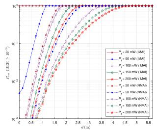
**FIGURE 11.** Outage probability versus the horizontal distance of the desired user from the AP for different transmit powers. MAI represents the case where the three other users are located at the same position at the room center. The three interferers and the desired user are oriented randomly at their positions. Only the LOS path is taken into consideration.
