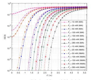
**FIGURE 10.** BER versus the horizontal distance *d* of the desired user from the AP for different transmit powers. MAI represents the case where the three other users are located at the same position at the room center. NMAI stands for no-MAI. Only the LOS path is taken into consideration.
