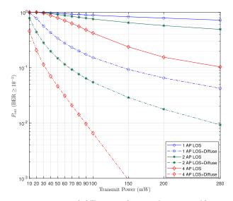
**FIGURE 18.** Outage probability versus the transmit power  $P_t$  with randomly moving and oriented desired user and interferers for the cases of one, two, and four APs based on the ORWP mobility model. Two cases of LOS and LOS+ 1<sup>st</sup>-order reflections are considered.
