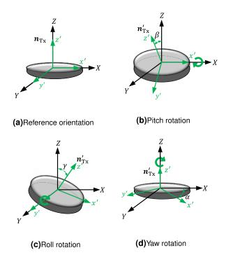
**FIGURE 4.** Orientations of a Tx: (a) reference orientation, when the reference coordinate system XYZ and the actual Tx coordinate system x'y'z' are aligned, (b) Pitch rotation, the Tx rotation around the X axis with angle  $\beta$ , (c) Roll rotation, the Tx rotation around the Y axis with angle  $\gamma$ , (d) Yaw rotation, the Tx rotation around the Z axis with angle  $\alpha$ .
