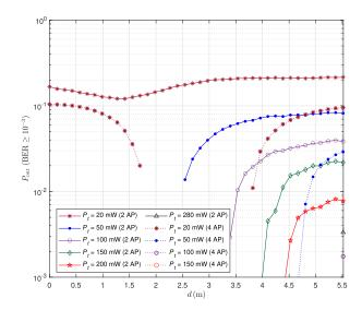
**FIGURE 17.** Outage probability versus the horizontal distance of the desired user from the center of the room for the 2 and 4 AP configurations for the case of NMAI. The desired user is oriented randomly at each position. LOS+1<sup>st</sup>-order reflections are considered.
