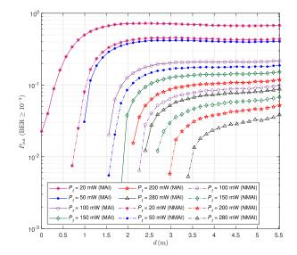
**FIGURE 14.** Outage probability versus the horizontal distance of the desired user from the AP, taking into account LOS and 1<sup>st</sup>-order reflections. The three interferers are randomly moving and oriented based on the ORWP mobility model inside the room; the desired user is randomly oriented at each position.
