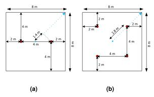
**FIGURE 15.** Arrangements of APs on the ceiling for the room size  $(8 \times 8 \times 3) \text{ m}^3$ : (a) case of 2 APs, (b) 4 APs. Here, dotted blue line represents the horizontal distance *d* from the center of the room.
