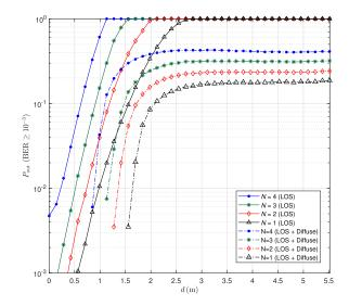
**FIGURE 13.** Outage probability versus the horizontal distance of the desired user from the AP for different numbers of users *N*. Interferers are located at the same position at the room center.  $P_t = 50$  mW. The three interferers and the desired user are oriented randomly at their positions.
