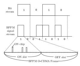
FIGURE 5. Example of frame structure of BPPM O-CDMA signaling.
