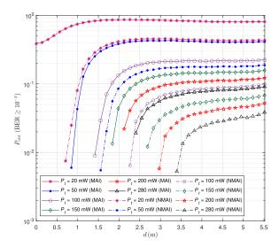
**FIGURE 12.** Outage probability versus the horizontal distance of the desired user from the AP, taking into account LOS and 1<sup>st</sup>-order reflections. MAI represents the case where the three other users are located at the same position at the room center. The three interferers and the desired user are oriented randomly at their positions.
