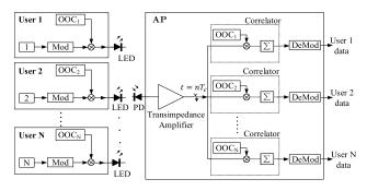
**FIGURE 6.** Block diagram of the proposed O-CDMA based extra-WBAN system; Blocks Mod and DeMod stand for modulator and demodulator. Signal sampling at the trans-impedance amplifier output is done at sampling period of *T*<sub>c</sub>, the chip duration.
