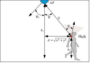
**FIGURE 2.** Illustration of a typical LOS link configuration between a CN and the AP. *x* and *y* represent the coordinates of the hub with respect to the room center, i.e., the AP position.
