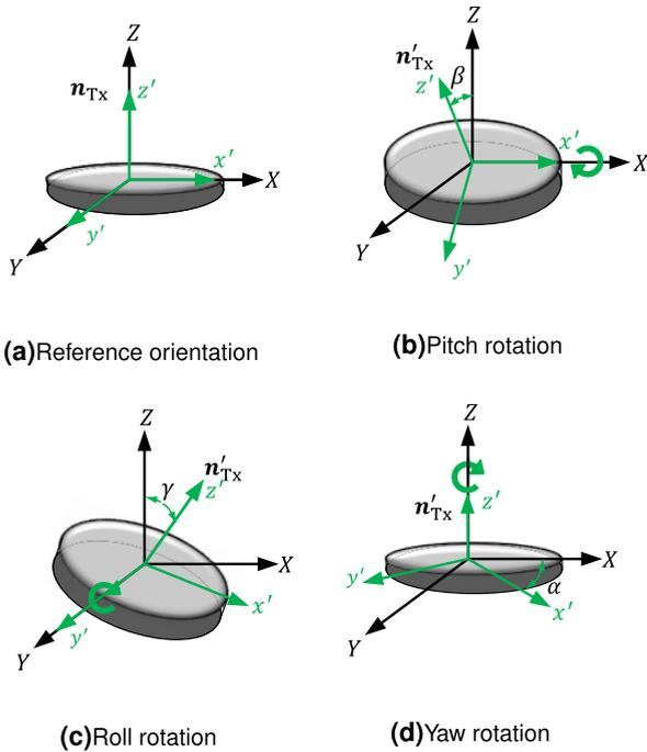
**FIGURE 4.** Orientations of a Tx: (a) reference orientation, when the reference coordinate system  $XYZ$  and the actual Tx coordinate system  $x'y'z'$  are aligned, (b) Pitch rotation, the Tx rotation around the  $X$  axis with angle  $\beta$ , (c) Roll rotation, the Tx rotation around the  $Y$  axis with angle  $\gamma$ , (d) Yaw rotation, the Tx rotation around the  $Z$  axis with angle  $\alpha$ .
