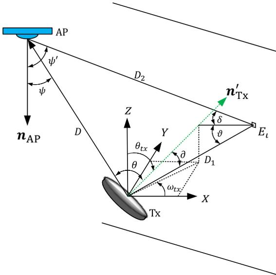
**FIGURE 3.** LOS and diffuse link with randomly oriented Tx. Here,  $\theta_{tx}$  denotes the elevation angle,  $\omega_{tx}$  is the azimuth angle, and  $n_{AP}$  and  $n'_{Tx}$  stand for the normal vectors corresponding to the AP and Rx, respectively.
