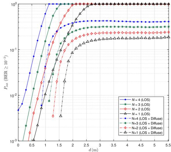
**FIGURE 13.** Outage probability versus the horizontal distance of the desired user from the AP for different numbers of users  $N$ . Interferers are located at the same position at the room center.  $P_t = 50$  mW. The three interferers and the desired user are oriented randomly at their positions.
