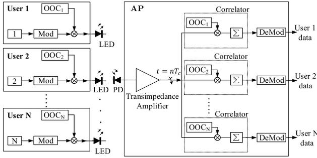
**FIGURE 6.** Block diagram of the proposed O-CDMA based extra-WBAN system; Blocks Mod and DeMod stand for modulator and demodulator. Signal sampling at the trans-impedance amplifier output is done at sampling period of  $T_c$ , the chip duration.
