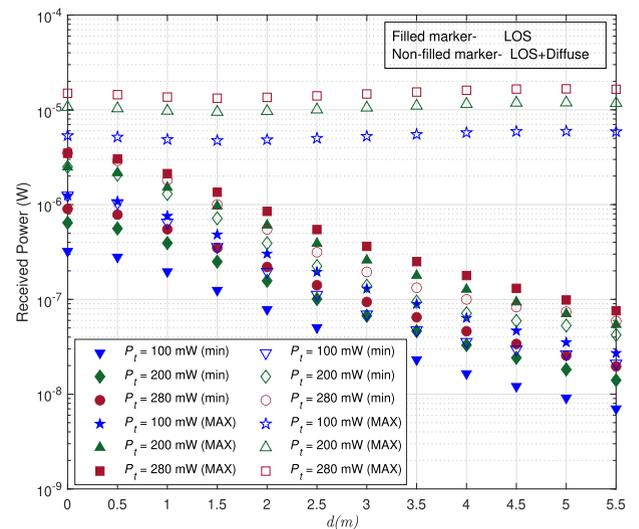
**FIGURE 8. Impact of Tx orientation on the minimum (min) and maximum (MAX) detectable received power for distances  $d$  from the room center. LOS and LOS+1<sup>st</sup>-order reflections are taken into consideration.**
