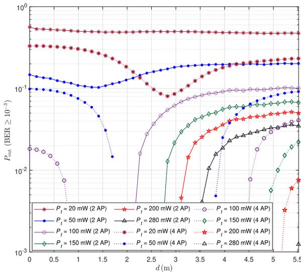
**FIGURE 16.** Outage probability versus the horizontal distance of the desired user from the center of the room for the 2 and 4 AP configurations, considering LOS+1<sup>st</sup>-order reflections. Three randomly moving and oriented interferers based on the ORWP mobility model; randomly oriented desired user at each position.
