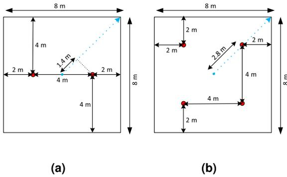
**FIGURE 15.** Arrangements of APs on the ceiling for the room size  $(8 \times 8 \times 3) \text{ m}^3$ : (a) case of 2 APs, (b) 4 APs. Here, dotted blue line represents the horizontal distance  $d$  from the center of the room.
