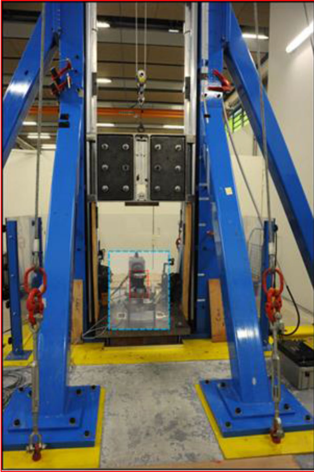
Figure 6. Photo of the drop tower testing equipment. The zone boxed in blue shows the sample and the interface parts (see details in Figures 7 and 8).
