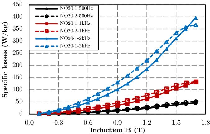
**Fig. 3.** Magnetic losses of NO20 at high frequency.
