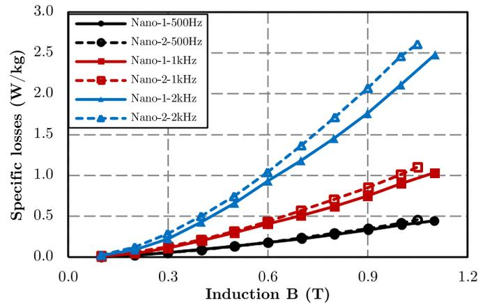
**Fig. 4.** Magnetic losses of nanocrystalline at high frequency.
