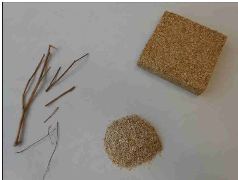
Figure 4. Photograph of the coriander straw used as raw material, of the 7.5 mm milled straw and of the insulation block made from it (from left to right)
