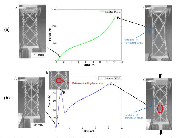
**Figure 3.** Tensile stress-strain response of (a) the BCC-Z with vertical struts substituted by sinusoidal corrugated struts, and (b) the designed structure with a « whistle-blower » behavior. Images taken at different strain increments are shown to illustrate the behavior of the structures at key steps.
