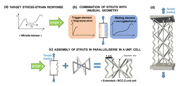
**Figure 2.** Summary of the design approach strategy. (a) Target stress-strain tensile response. (b) Step1: combination of struts with unusual geometries exhibiting elementary behavior. (c) Step 2: Introduction of struts with unusual geometries in parallel or in series into unit cell (BCC-Z here) to produce the "Extended" BCC-Z unit cell designed to generate a "Whistle-blower" mechanical behavior. (d) Final design of the tensile specimens for validation.
