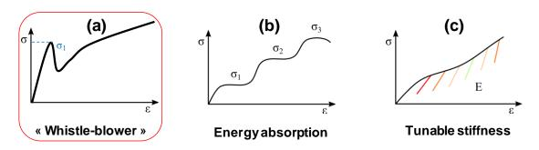
**Figure 1.** Examples of unusual stress-strain response. (a) "Whistle-blower" mechanical behavior. Stress-strain response (b) with multiple stress plateau for energy absorption and (c) for tunable stiffness.
