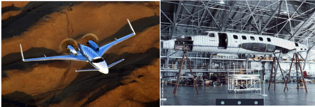
Fig. 21. Left: Beechcraft Starship NC 51 in flight, Right: Fuselage under construction (from [150]).
