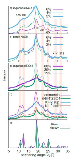
Figure 6 a-d) X-ray diffraction profiles of freeze-dried xylans after subtraction of air scattering
