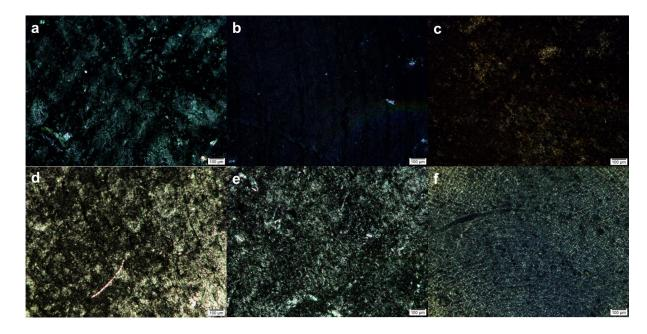
**Figure 5** Cross-polarized microscopic images of xylan films (a) H1-F, (b) H8-F, (c) H11-F,(d) H5-NF, (e) H7-NF, and (f) H14-NF. Scale bar =  $100 \mu m$ . Note: "F" means sample formed an integral film; "NF" means sample formed broken films.
