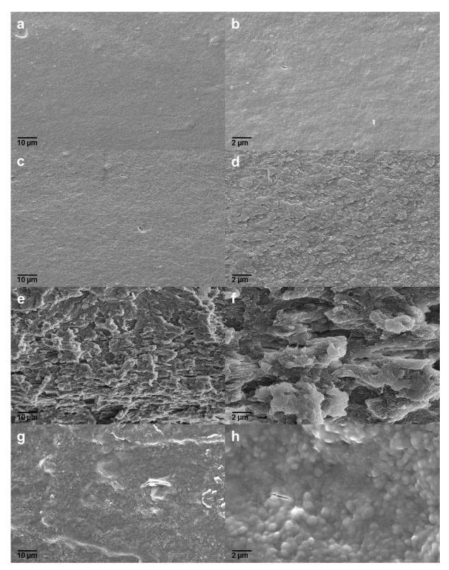
Figure 4 SEM images of the film cross-section (from the natural cracking position for broken
