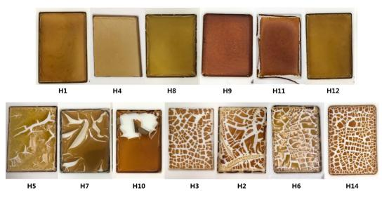
**Figure 2** The films casted in Teflon molds.
