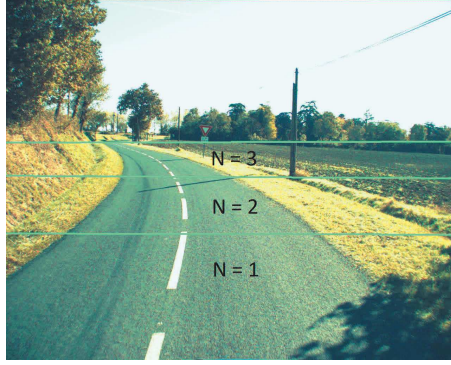
Fig. 3 The adopted ground truth for lane simulation with N = 3 hyperboles.
