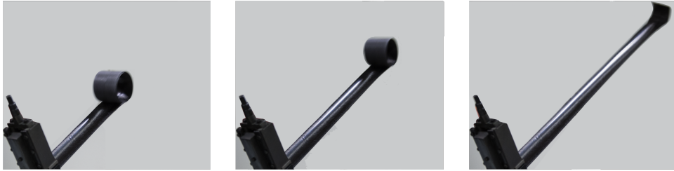
Figure 1: Dynamic deployment of a bistable tape spring. From a coiled configuration to a deployed straight one, from left to right.
