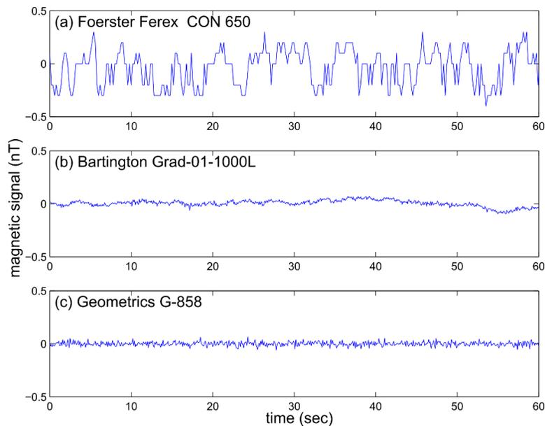
**Figure 2.** Comparison of stationary measurements collected with three different magnetometer sensors over one minute: (a) Foerster Ferex Con650; (b) Bartington Grad-01-1000L; (c) Geometrics G-858 (data courtesy of Geocarta SAS, Paris, France).
